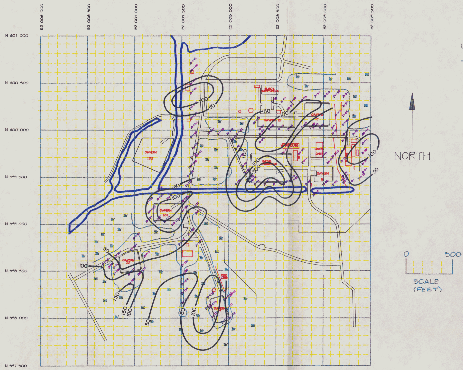
FIGURE 3.1-5 ELECTROMAGNETIC TERRAIN CONDUCTIVITY RESULTS - SHALLOW DEPTH OF INVESTIGATION BAYOU CHOCTAW SPR SITE IBERVILLE PARISH, LOUISIANA Source: ECT, 1993.
